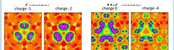
Comparison of the values of g-factor extracted from the operando ESR experiment and that obtained from the calculations performed for the system with various vacancies at many charge levels enables to characterize the mesoscale samples and correlate their transport properties with the existence of the specific defects.
