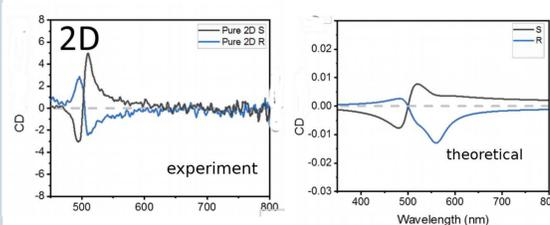
Comparison of the experimental and theoretical spectra of the circular dichroism in pure 2D structures with chiral molecules. Simulations were done with the **time-dependent DFT (TDDFT)** using the Yambo code.
